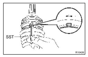
(e) Assemble the boot clamps to both boots.
